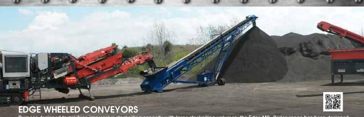
Purpose designed to produce impressive stockpiling capacity with large stockpiling volumes, the Edge MS- Series range has been designed with productivity, mobility and minimizing operators" cost in mind. The MS-Series wheeled stacker conveyors are designed and manufactured to deal with increased production capacity and to facilitate larger stockpiles. The MS-Series stacker conveyors are the most cost effective and efficient way of stockpiling material on the market today.
